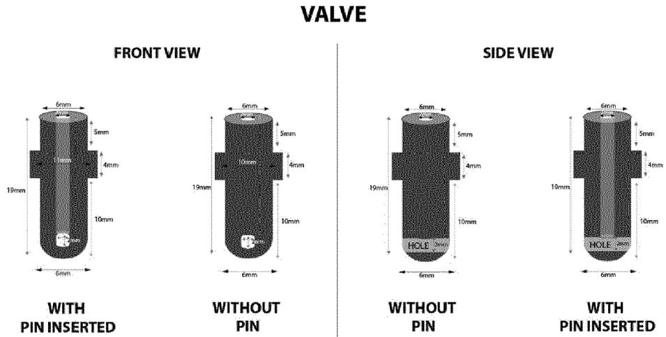
Fig. 4: Schematic Front and Side View of a Dual Function Valve with and without Inserted Pin
