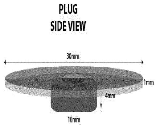
Fig. 3(a): Schematic Perspective Side View of an anchor plug
